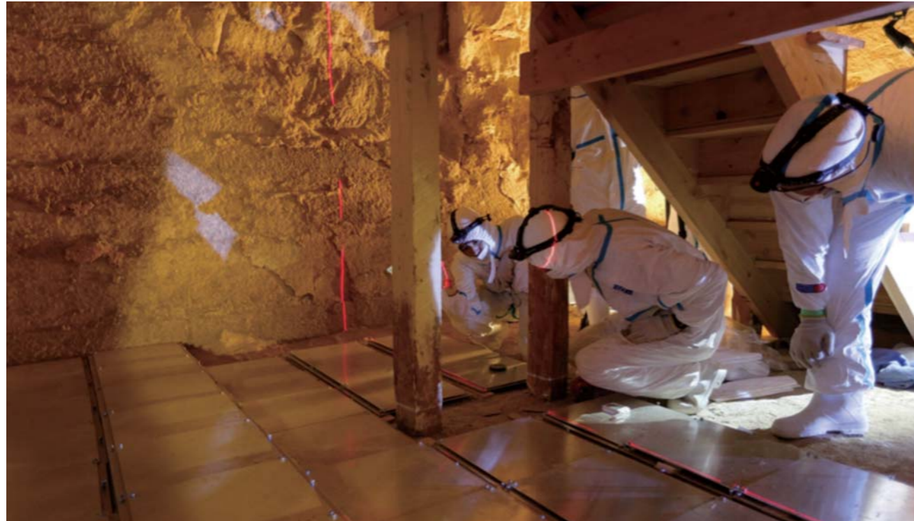
Installation of nuclear emulsion detectors inside the Bent Pyramid at the Dahshur necropolis in Egypt. Aluminum plates, which fix nuclear emulsions, were placed horizontally on the ground inside the lower chamber to measure cosmic rays to validate imaging of the upper chamber.
